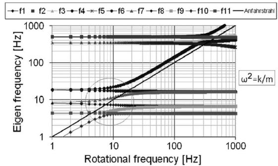
Fig. 5. Calculated diagram of flywheel rotor eigenfrequencies.
