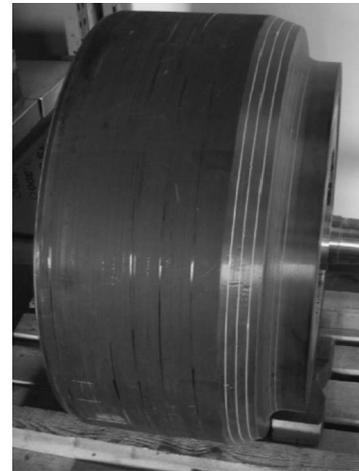
Fig. 3. Multirim flywheel rotor.
