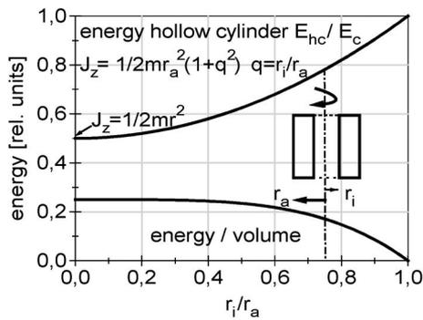
Fig. 7. Geometry and energy factors of a rotating hollow cylinder.
