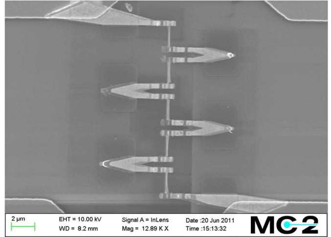
Fig. 2. SEM image of half of an array consisting of five absorbers and ten SIN tunnel junctions. One can see five absorbers of bolometers as narrow strips in the center. SIN tunnel junctions (horizontal, center) are connected to the antenna terminal at its edges through a planar capacitor that provides a parallel connection of bolometers to the antenna port.
