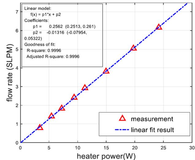
(b) Flow rate versus heater power
